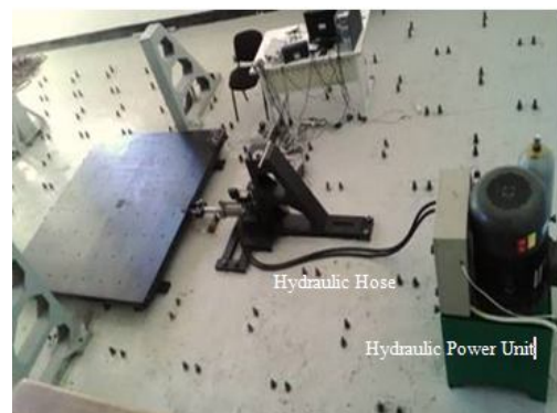
Fig. 3. Setting of shaking table, reaction frame and actuator cylinder on concrete floor
